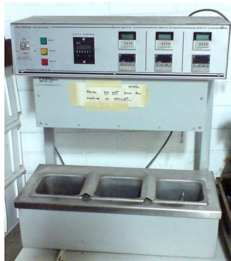
A very early PCR machine Samples moved mechanically
