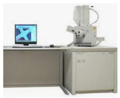
Philips XL 30 Scanning Electron Microscope
